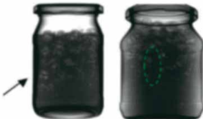
The enhanced inspection system (right) of the Rayon X3 allows to detect thin contaminants (Rayonics).
